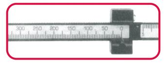
To increase weight values, move the poise to the left and line up the indicator with the desired graduation. Always make sure the pawl is seated in the notch.
