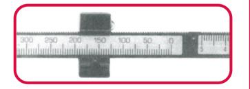
Do not attempt to set the large poise at any position except firmly seated in a notch. Always use the small poise for weight values between the 5 grain increments of the large poise.
